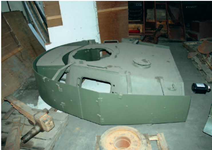
➤ The turret is painted with a green anti rust paint. The « Schürzen » have been fully rebuilt.
