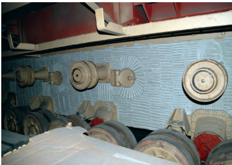
➤ After having been totally stripped down, the tank got its Zimmerit coating again. The latter is made of tile cement.
